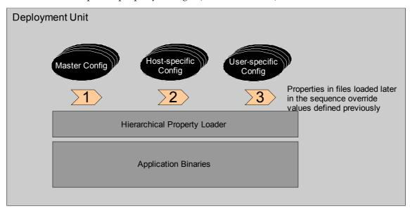
Illustration 2: Structure of deployment unit with a HIERARCHICAL PROPERTY LOADER
